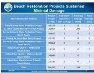
This was my favorite damage table. On its face, its rather stupid – a whole bunch of zeros. But what does it tell us? It shows indisputable evidence, that where the coast was protected by a beach restoration project, there was essentially no significant damage. The one structure damaged at a project, was the Jacksonville Beach pier, which was seaward of the project. And the armoring damage was some relatively minor damage to a very old wall at St. Augustine Beach.
