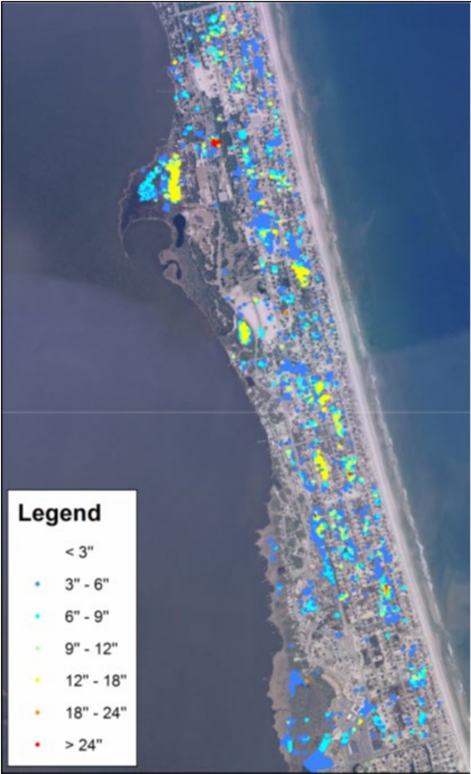
Flooding during an 8" rainfall event
