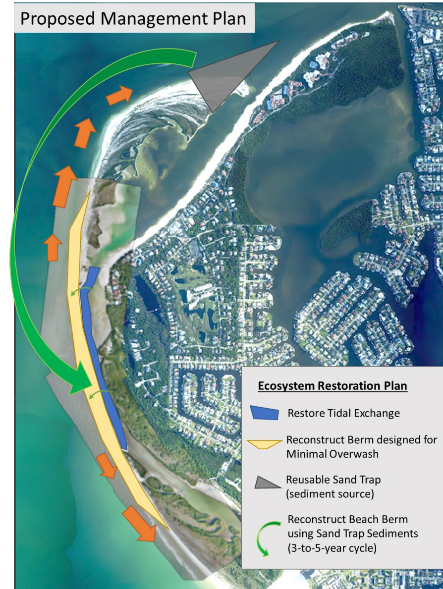
Schematic of nature-based restoration elements
