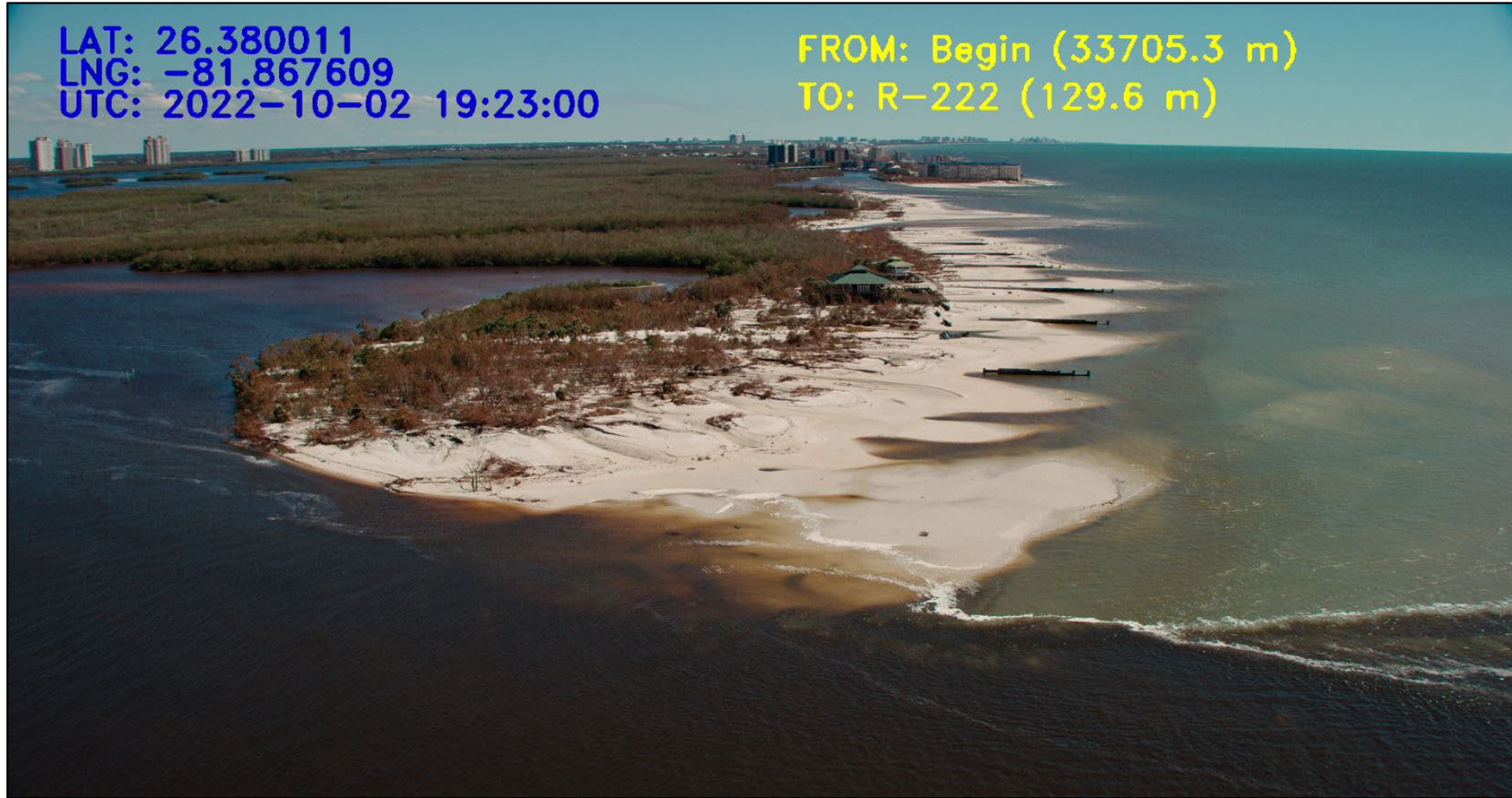
Hurricane Ian's beach and dune damages (Condition IV), Big Hickory Island (R-222) video photo by Camera Copters and Active Camera Systems
