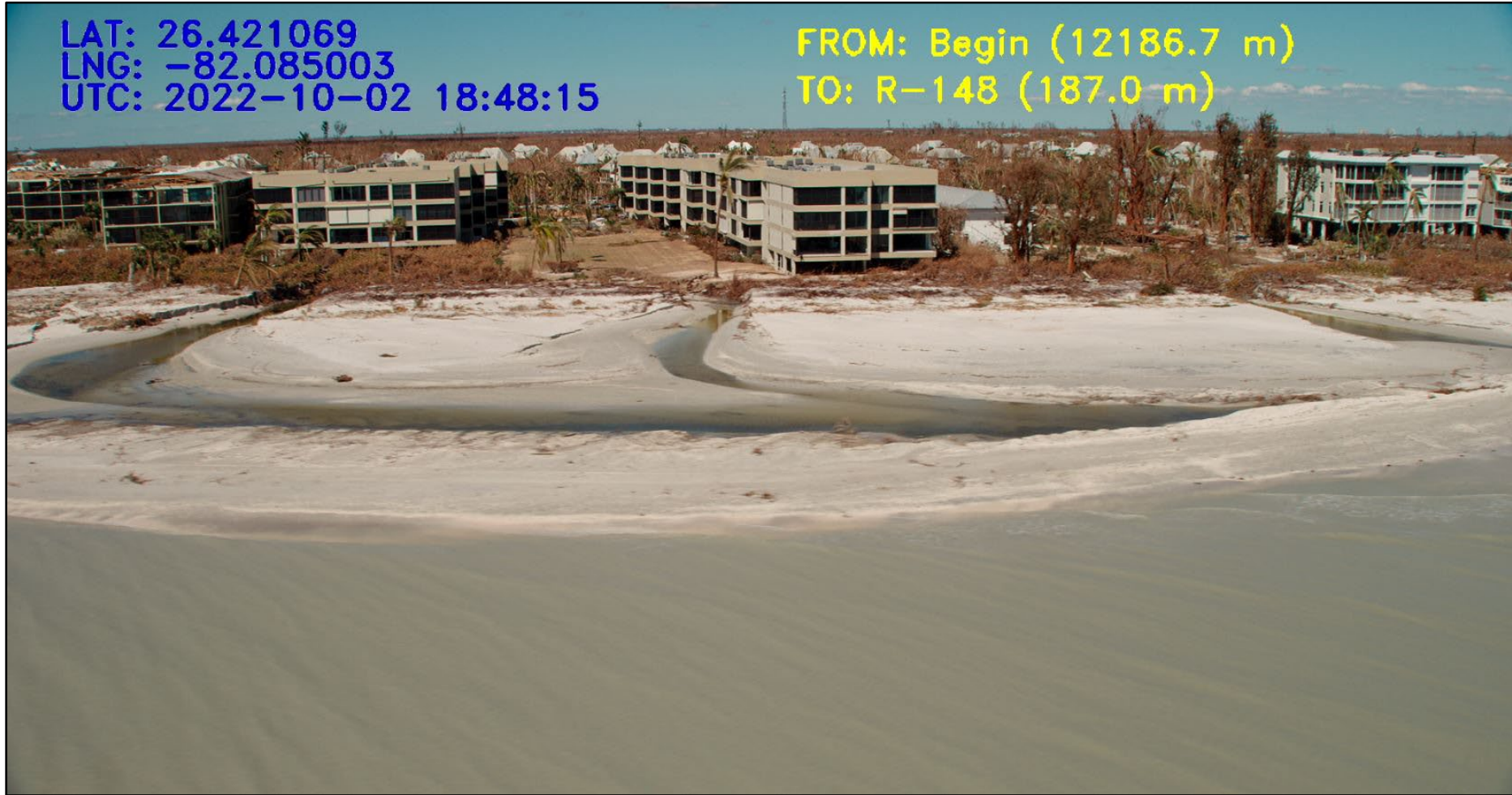
Hurricane Ian's beach and dune damages (Condition IV) on Sanibel Island (R-148), video photo by Camera Copters and Active Camera Systems
