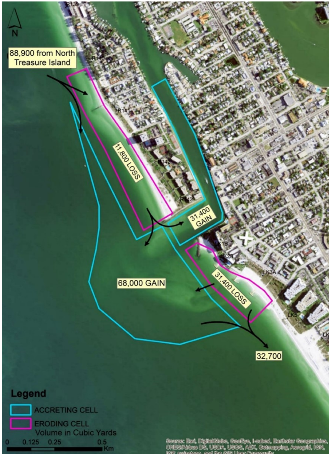
Figure 3. Annualized sediment budget at Blind Pass based on field data collected from October 2010 to June 2014 (aerial photography 2014; Wang et al., 2016).
